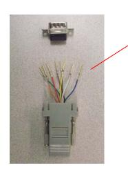
Insert wires into correct pins as described in the table. Pin numbers are engraved on the back of the connector.
