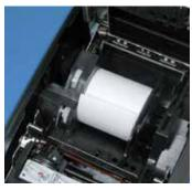
Drop and Print Paper Loading with Built-In Paper Width Selector
