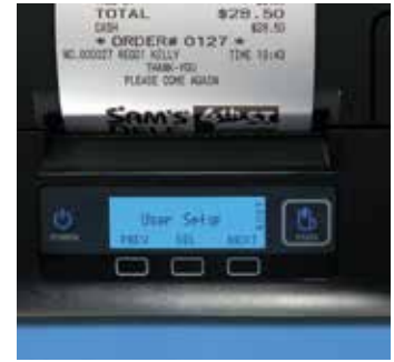
Liquid Crystal Display Guides the Operator Through Setup and Option Selections
