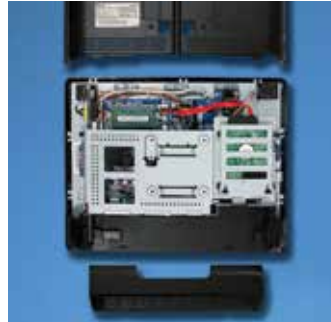
Tool-Free Access to RAM Optimizes Serviceability
