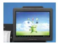
Use the adjustable 9.7" color touch screen for operating the POS solution by touch.
