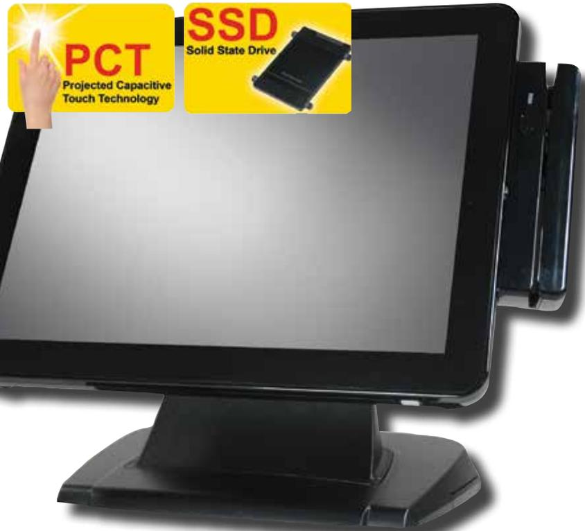
For extraordinary reliability, the SPT-4846 includes both projective capacitive touch and a choice of solid state or hard disk drives. Powered by an Intel Celeron **dual-core fanless** processor and designed with a true flat touch panel, the SPT-4845 provides superior spill and dust resistance that ensures optimum performance in harsh retail and food service environments.
