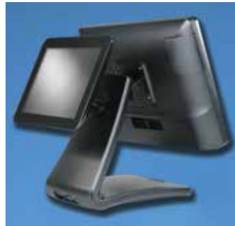
Optional Integrated 9.7" and 15" Rear LCD Customer Displays
