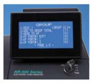
**Operator Display** The easy-to-read, blue backit, 192 x 64 graphic LCD operator screen identifies each item as it is entered.
