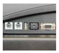
**Connector Panel** A combination of three serial ports and one USB port are available to support popular off-the-shelf POS peripherals.
